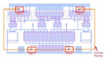
Fig. 1: The routing layers of a manual comparator layout.
