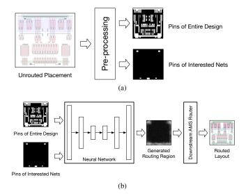
Fig. 8: Inference phase. (a) Data pre-processing. (b) Model inference.
