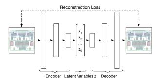
Fig. 4: Architecture of an autoencoder.
