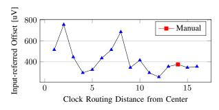
Fig. 3: Comparator input-referred offset experiment results.
