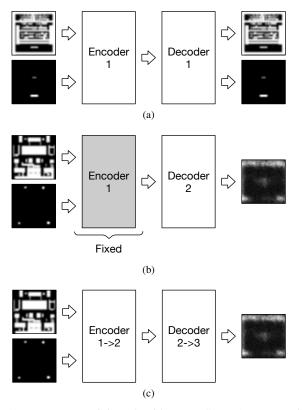
Fig. 11: Tree-stage training algorithm. (a) Stage 1: unsupervised initial feature extraction. (b) Stage 2: supervised decoder training.(c) Stage 3: model fine-tune with reduced learning rate.
